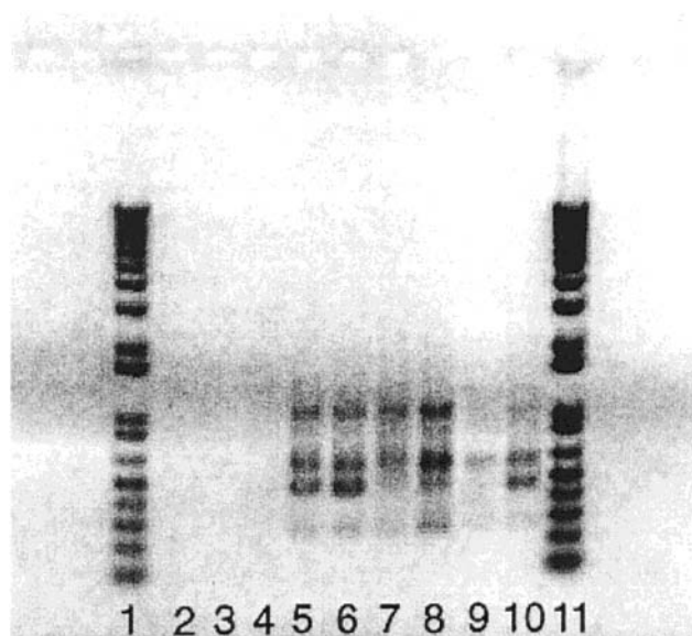
Figure 5. Slab gel electrophoretic separation of the 1 kilobase pair PLUS DNA standard relative to the separation of four grape plant varieties as well as three different Chardonnay samples in 0.5% Trevigel-500 TAE buffer, pH 8.5, containing 10 \mu g/mL of ethidium bromide intercalator, run at 100 V. Sample wells are indicated by an arrow. DNA fragment sizes are given in base pairs. Lane identification: (1) 1 kbp DNA ladder PLUS standard, (2) blank, (3) blank, (4) negative control (contains all RAPD reagents but not genomic DNA), (5) Glebe '91 Chardonnay, (6) Glebe '86 Chardonnay, (7) Williamsburg Merlot, (8) Williamsburg Cabernet Sauvignon, (9) Williamsburg Cabernet Franc, (10) Williamsburg Chardonnay, and (11) 1 kbp DNA ladder PLUS standard.
